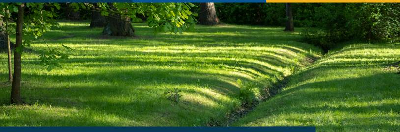
**Residential surface drainage** is the method of directing rainwater and runoff away from your home and property to prevent flooding, erosion and potential damage to your foundation. It involves creating a slope or channels on the ground to guide water away from your house towards a suitable drainage point, such as a storm drain or a lower point on your property.
